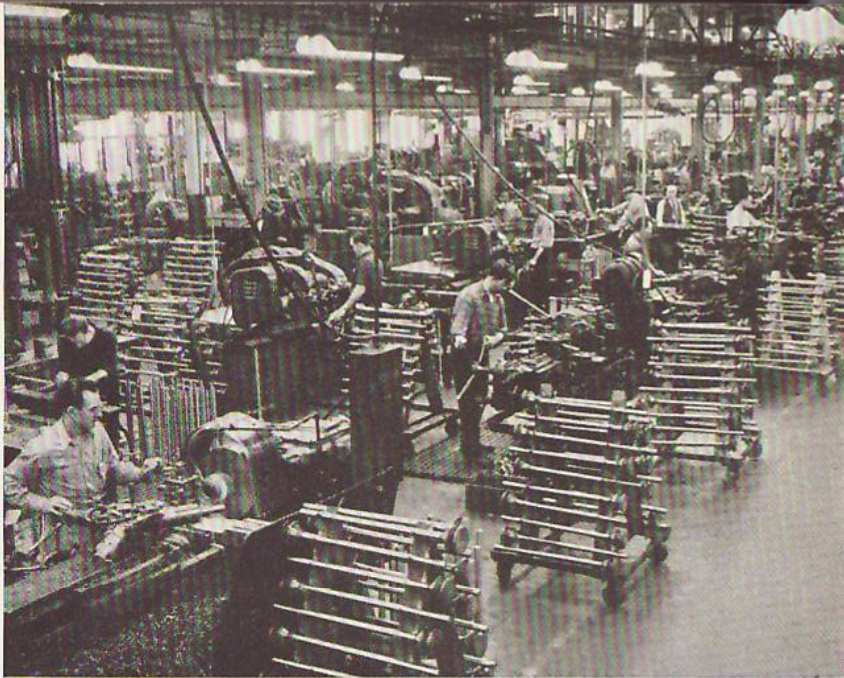
One of De Soto's jobs was machining the piston rods of the gun recoils.
