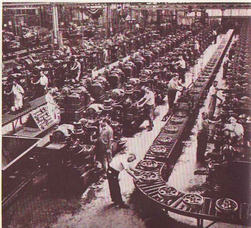
Herringbone final drive reduction gears passing down a line of gear shapers.
