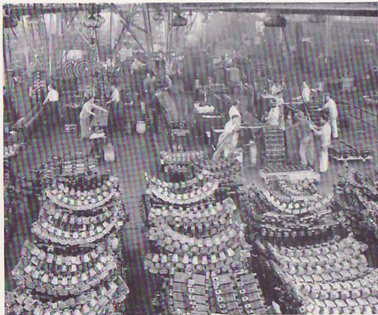
Assembling tank tracks. Tanks began with rubber shoes, were forced to shift to steel for lack of rubber.
