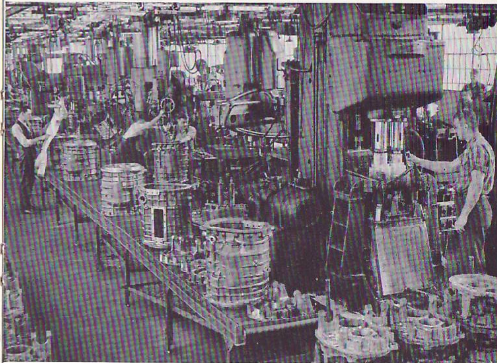
Tank transmission case machine line. Only heavy machining remained at the arsenal after expansion plans put many operations in other Chrysler plants.
