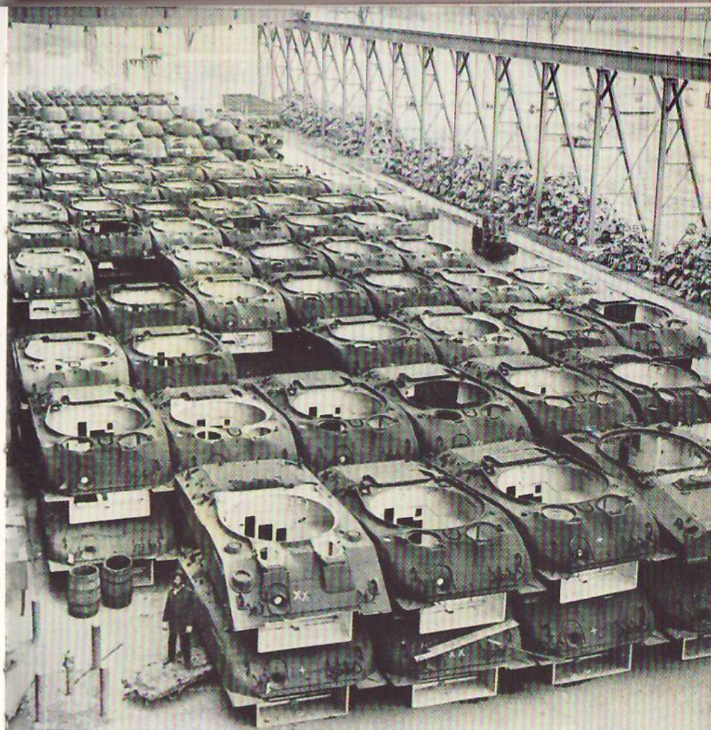
Sherman hulls, turrets and front end drive housings stored in the open at the arsenal, November, 1943.
