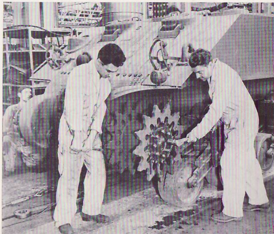
Adding the front drive sprockets which drive the tracks. The tank nears completion.
