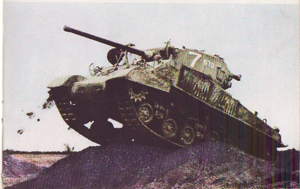
Testing the Chrysler Engineering-designed horizontal volute suspension at the proving grounds before production.
